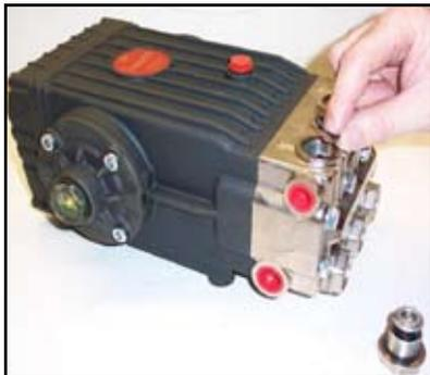
**Figure 4-4. Apply Grease and Install Valves**
