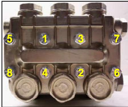
**Figure 4-17. Torque Sequence in "X" Pattern**
