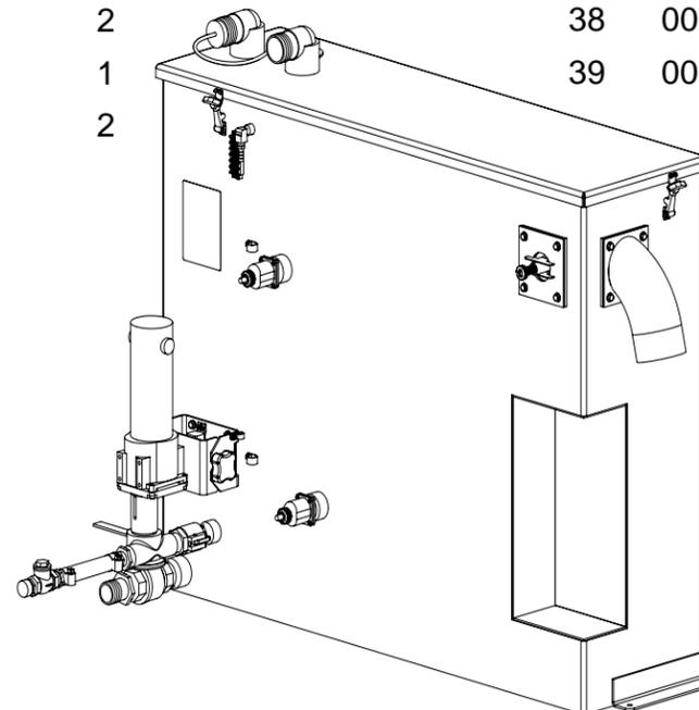
Figure 9-41. 100 Gallon Universal Recovery Tank Cover Assembly
