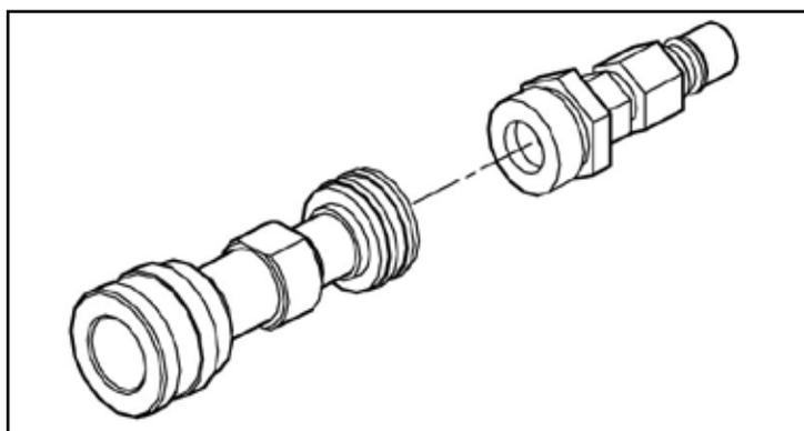
**Figure 4-19. Recirculation Fitting**
