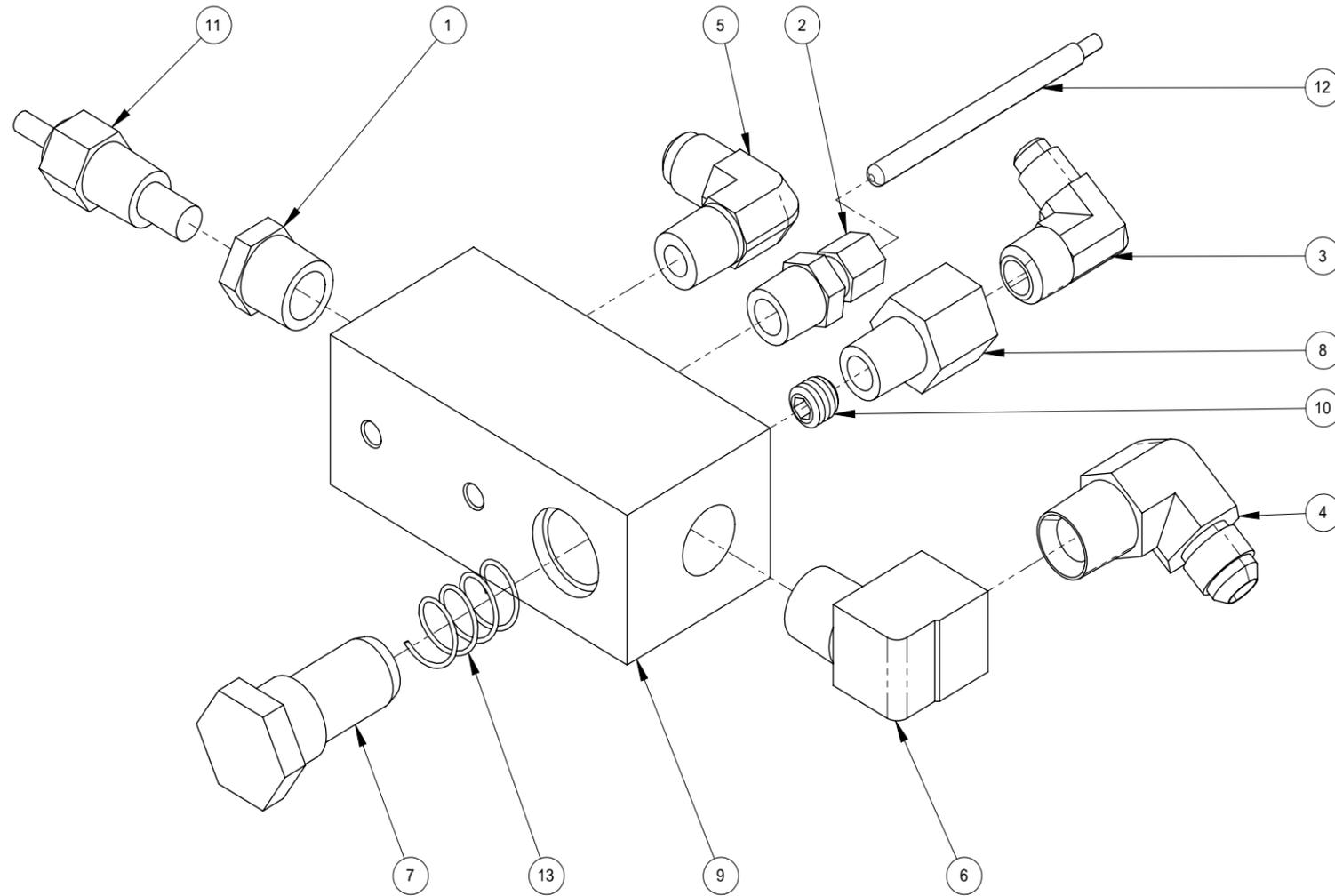
**Orifice Manifold Assembly Parts List**
