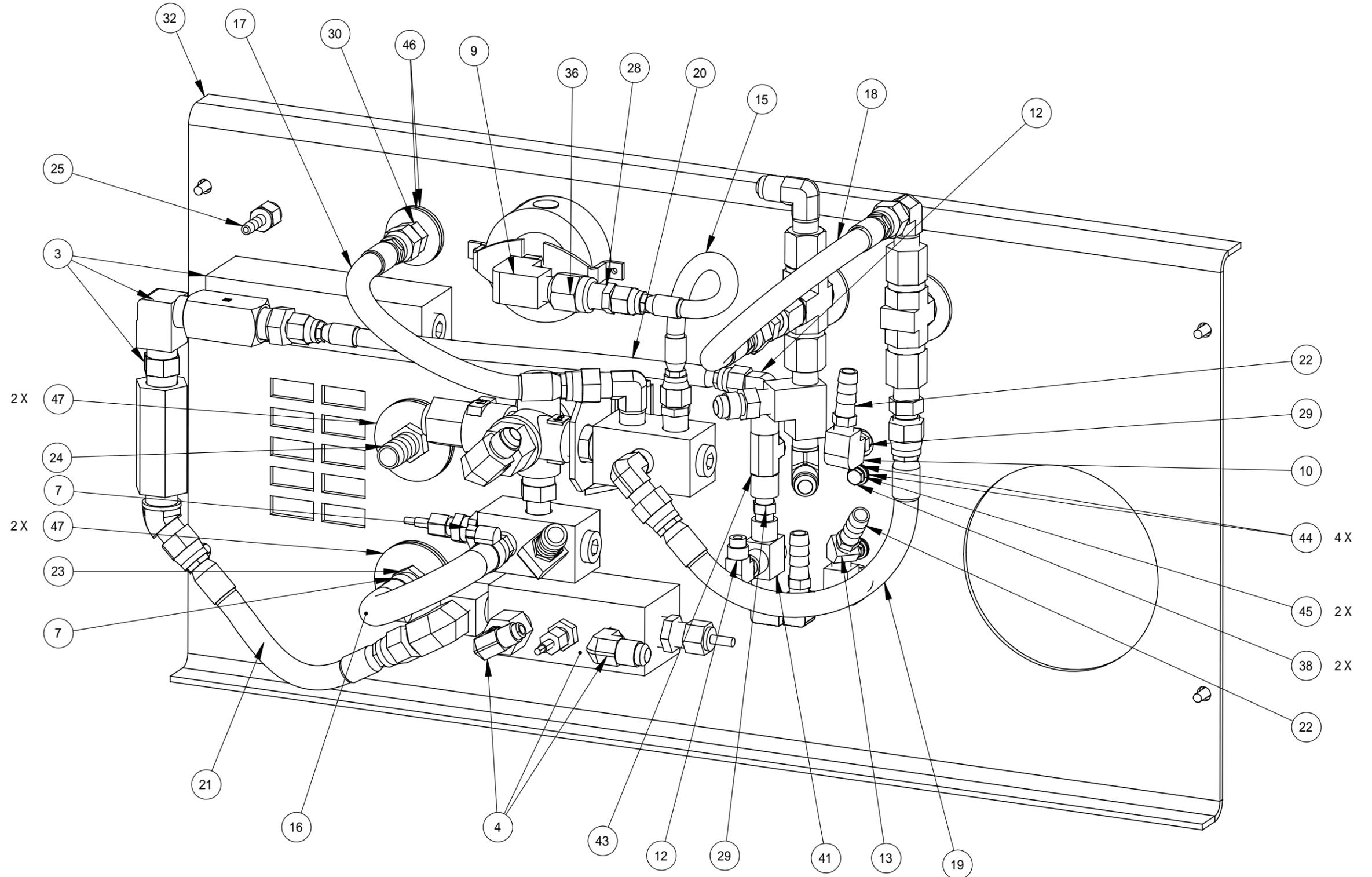
Figure 9-24. Lower Instrument Panel Assembly - View 3 of 3
