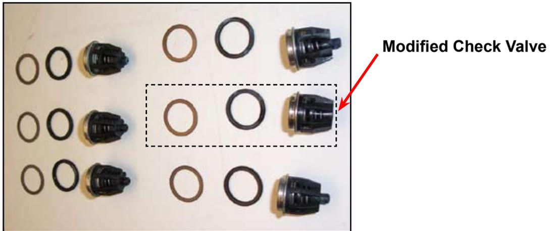
**Figure 4-3. Replace Center Inlet Check Valve With Modified Check Valve**
