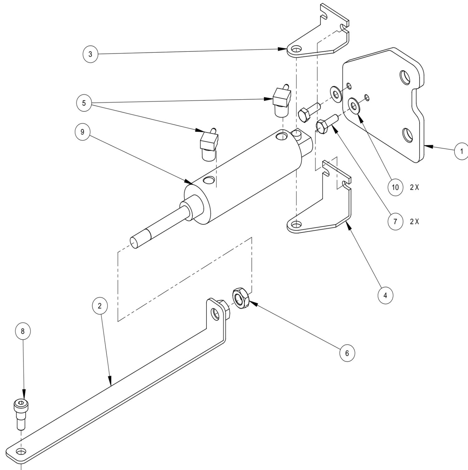
**Air Actuator Assembly Parts List**
