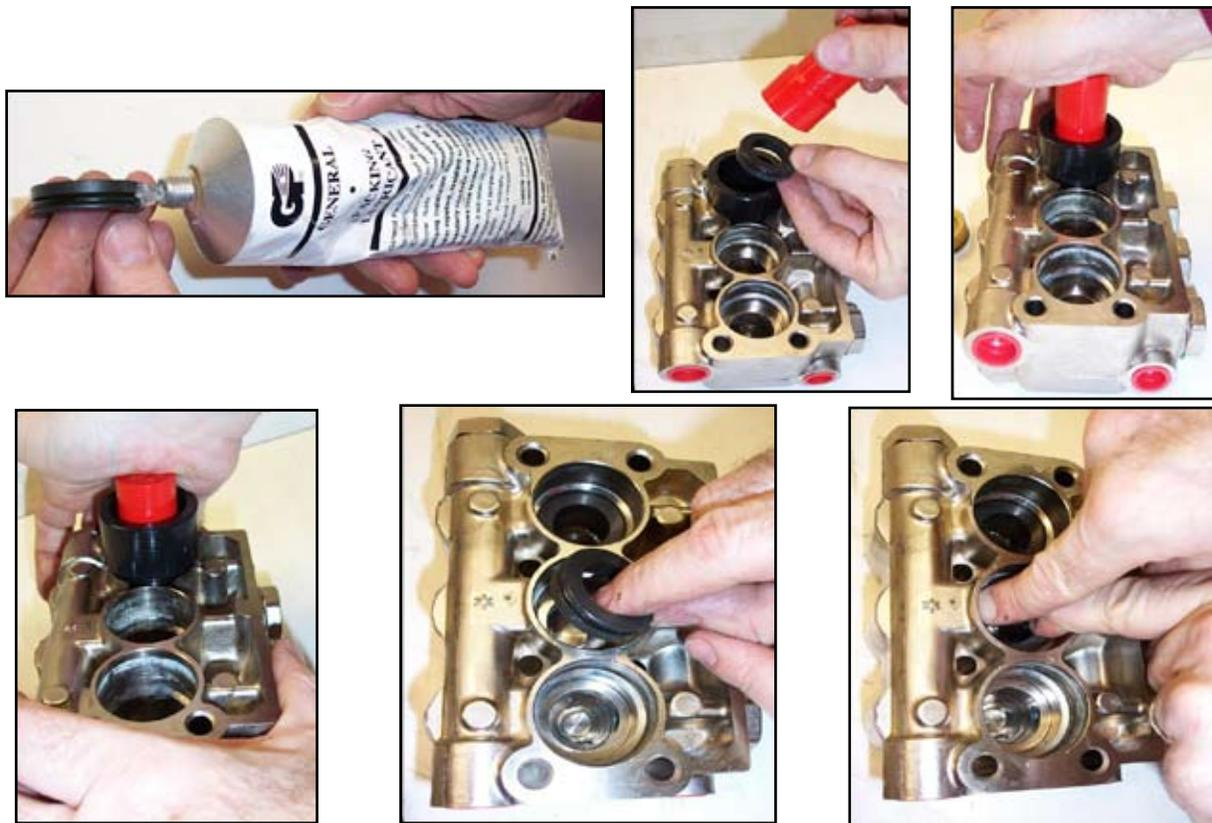
**Figure 4-13. Install Seal Assembly Using O-Ring Grease**
