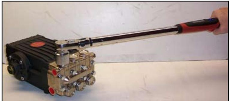
**Figure 4-5. Replace Valve Cap and Torque to 95 ft lbs**
