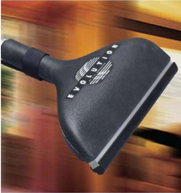
The Evolution Wand is truly the next evolution in wand design and performance. The Aluminum tube and Rotomolded head make it extremely lightweight which helps to reduce fatigue on the technician. The sealed Delrin® glides help the wand to be easily pushed across the carpet, and are tapered to keep a good seal on the fibers.
