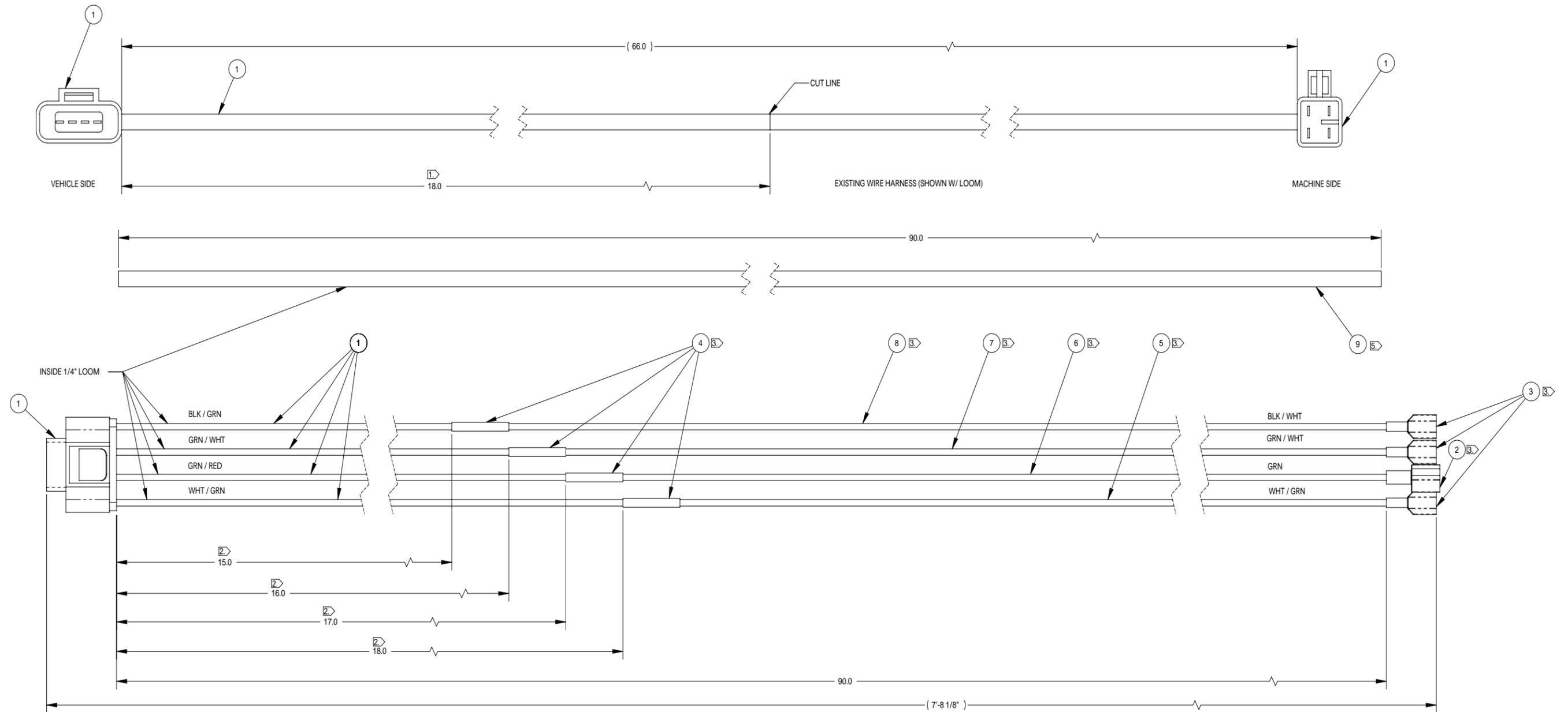
**Figure 7-6. Schematic of Wire Harness - Fuel Pump Manifold to Machine - View 2 of 2**
