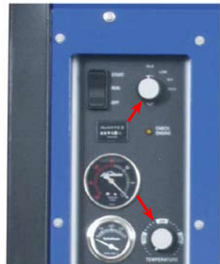
**Figure 5-5. Rotate Thermostat Dial and Select Engine rpm**
