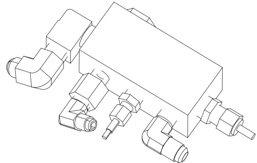
**Figure 9-27. Hi Pressure Out Manifold Assembly**
