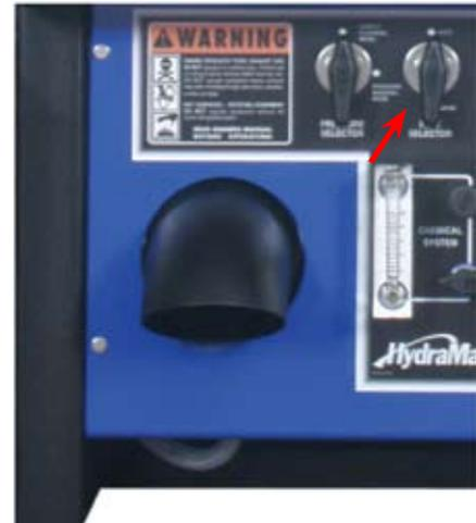
**Figure 5-4. Set Heat Selector Valve**
