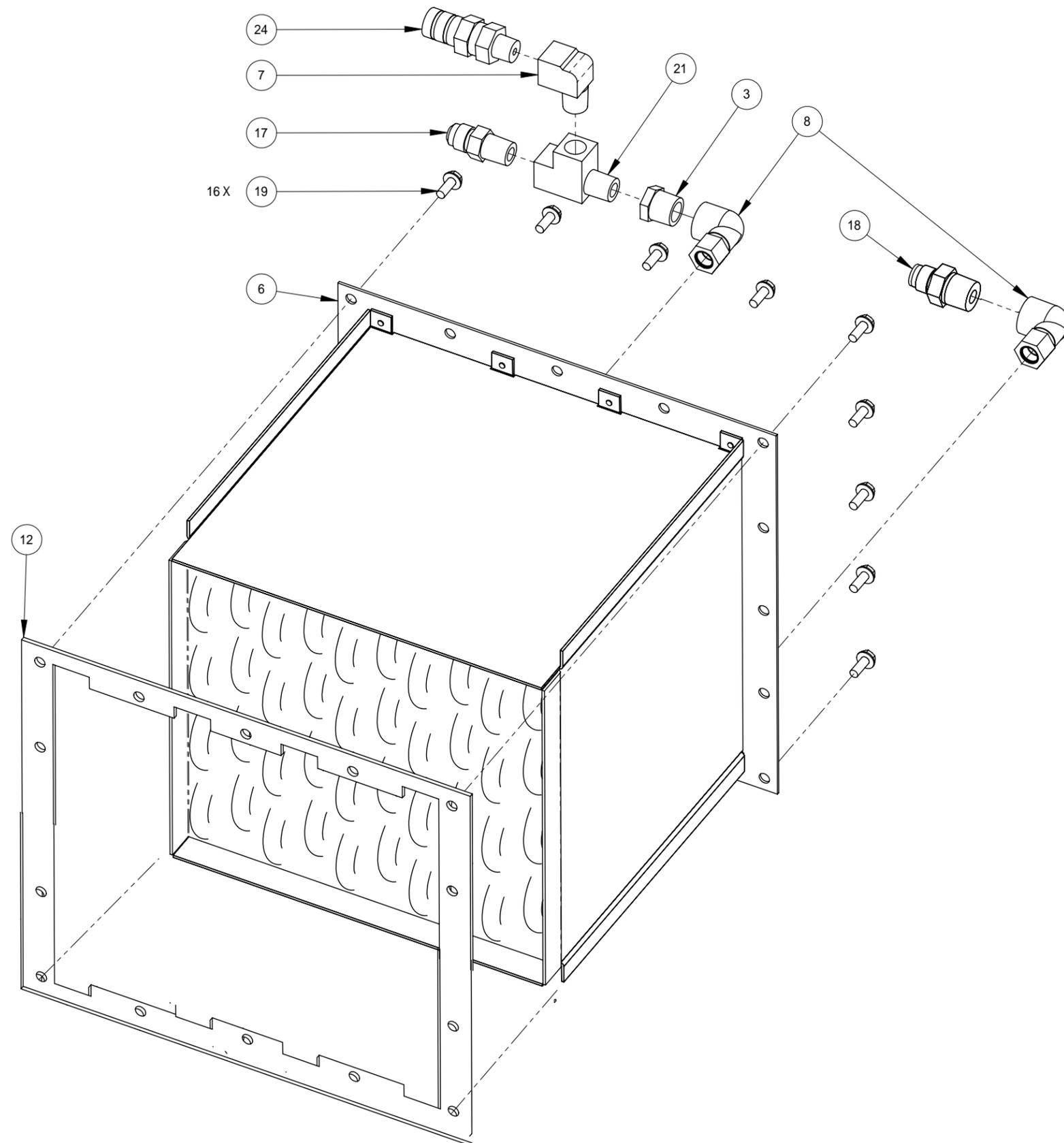
Figure 9-20. Blower Heat Exchanger Assembly - View 2 of 2
