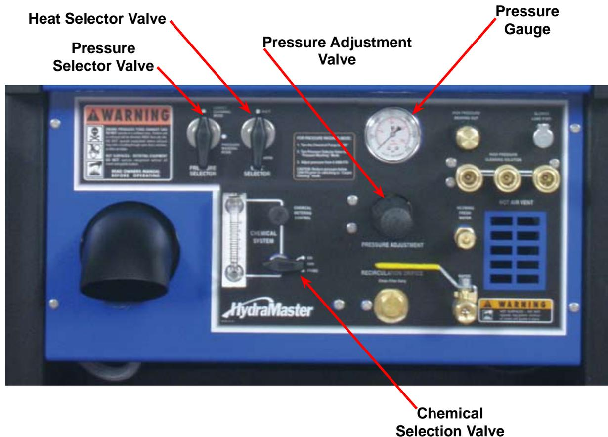
**Figure 5-2. Titan 875 Lower Dash Assembly**
