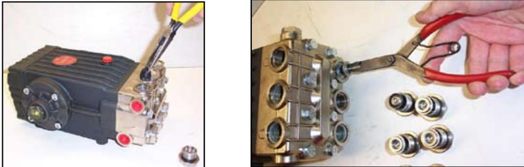
**Figure 4-1. Remove Valve Cap and Valve Assembly**
