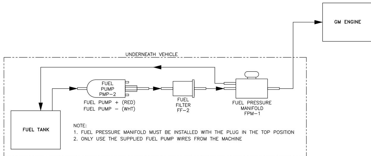
**Figure 2-1. Fuel Pump Diagram**
